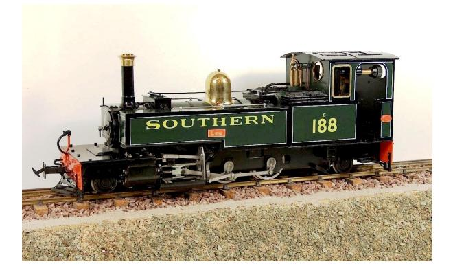
Lew was built in 1925 to a similar design to the previous Manning Wardle locomotives constructed for the Lynton & Barnstaple Railway, the main difference being a redesigned cab to eliminate a smoke trap, and give more room to the crew.
